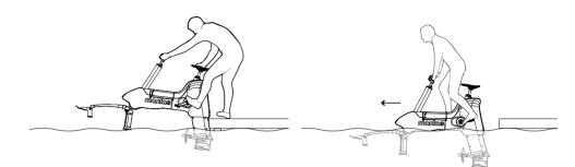
1. Place Hydrofoiler into the water at jetty edge.
