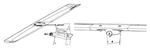
Attach the front tiller to the steering fork by tightening the countersunk screw into nylock nut (use 5 mm hex key).
