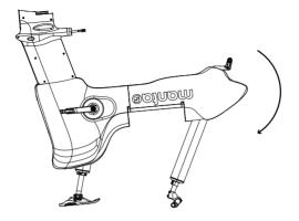
3. Attach rear foil using 6 mm hex key .
